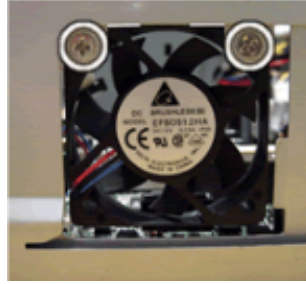
Fig. 17: Removing the auxiliary system fan
